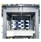
The high-performance robot palletizer PRINCIPAL-R, an articulated arm robot palletizing system, is always offered as customer-specific solution with well-known industrial robot manufacturers and STATEC BINDER know-how. Depending on the desired performance, different robot models are used. The gripper is also adapted to the respective application. A special feature of the PRINCIPAL-R is that it has been optimized for sling bags.
