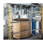
The semi-automatic Big Bag Filling Station enables the filling of Big Bags (FIBC) with one, two or four loops and Octabins with a filling weight from 500 kg to 1500 kg.
