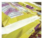
The patented bag closing system "Over Tape Bag Sealer" from STATEC BINDER seals woven polypropylene (PP) bags airtight. A woven PP tape is used for a reliable and secure closure. If necessary, the bags can also be additionally sewn. Both pillow bags and gusset bags can be securely closed. This sealing technology facilitates the handling of dusty products of the food and feed industry and odour-intensive products.
