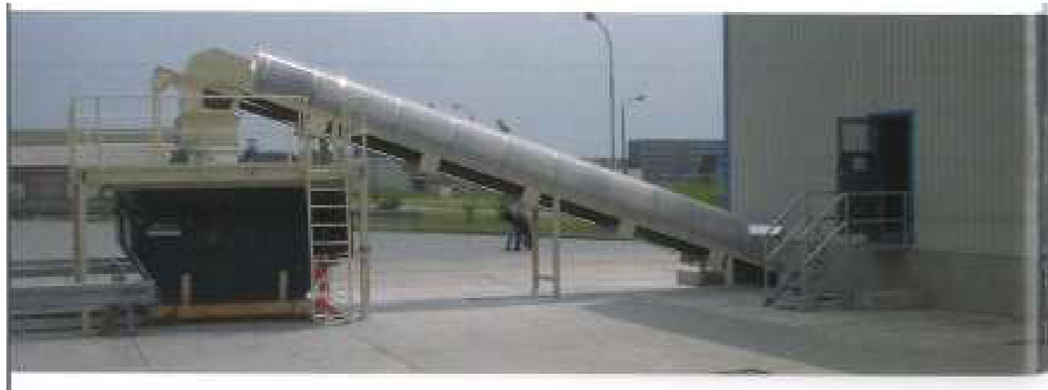
Cullet disposal: float glass coating
