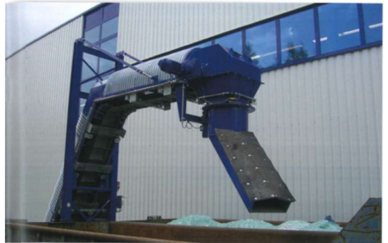
Cullet disposal: float glass cutting
